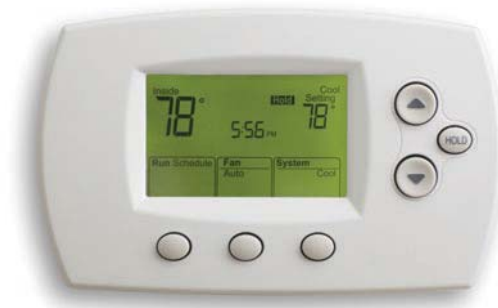
FIGURE 3: A thermostat can be used to control the heating and cooling systems in a home.
